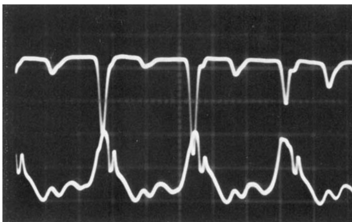
FIGURE 15. Dual-channel oscilloscope traces from a cold-wire-hot-wire pair sensor located at x/D = 0.6 at the transverse location where U/U_e \approx 0.10 . Upper trace is the temperature signal (inverted), and the lower trace is the u signal.
